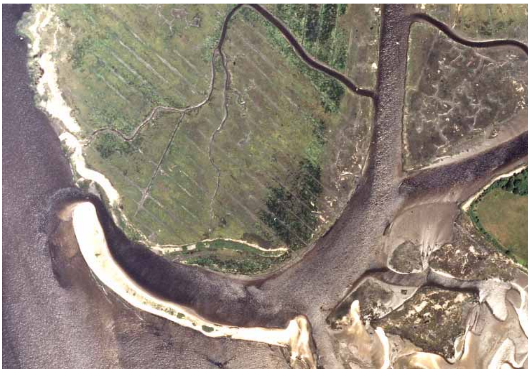
This aerial photo taken in Sept 2002 shows the contrast between ditched and unditched wetlands. Note the abundance of small ponds and meandering creeks on the marsh islands to the east and southeast of Great Island, which is heavily grid-ditched. The narrow strip of marsh on the southeast side of Great Island that contains numerous ponds and creeks is also unditched.
