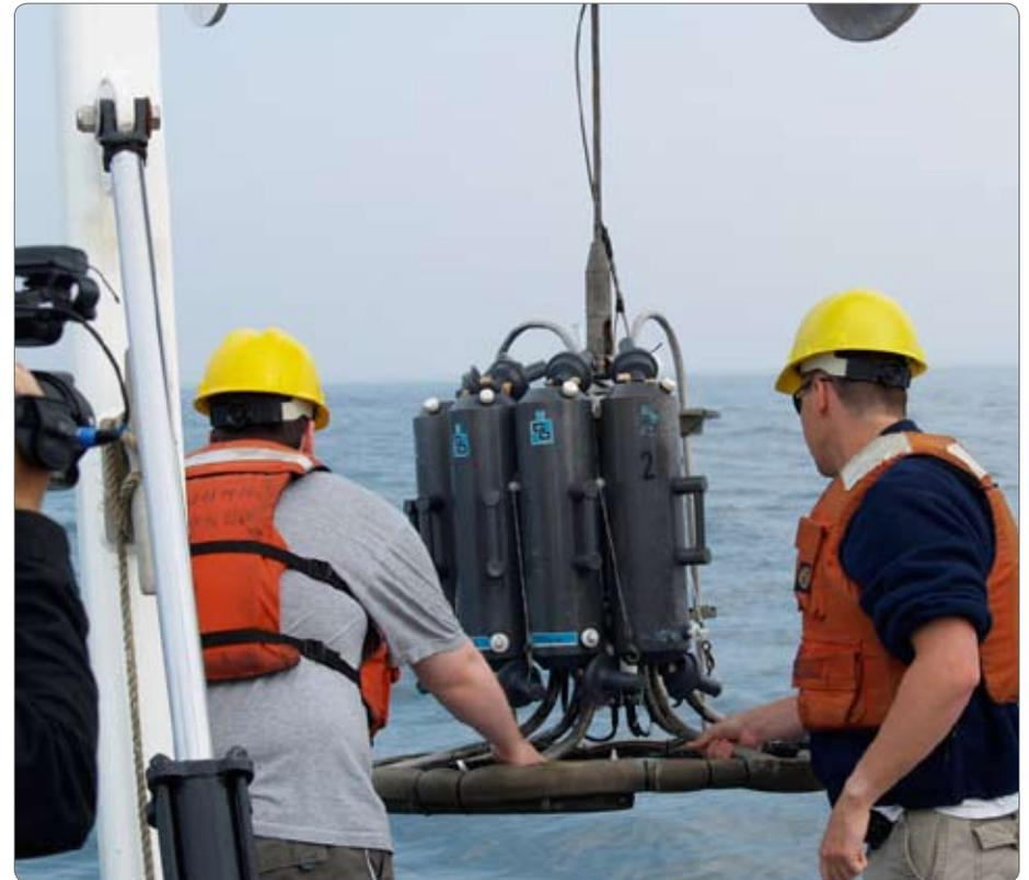
▲ **THE ROSETTE SAMPLER** is deployed off the stern of the *Dempsey* in the Race at the eastern end of Long Island Sound.
