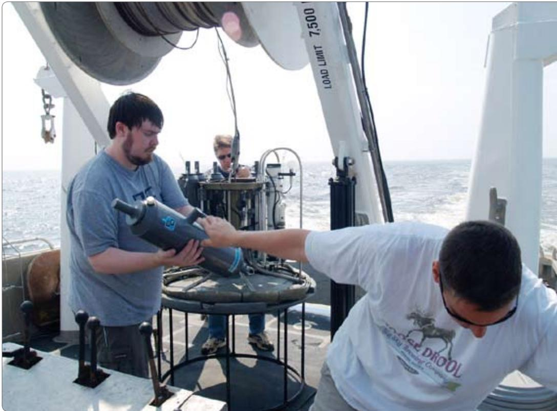
▲ **THE BOTTLE BRIGADE**, the field crew onboard the *Dempsey* passes Niskin bottles preparing the rosette to collect more samples. A total of 10 Niskin bottles can be mounted on the rosette allowing the field crew to collect samples at different depths.
