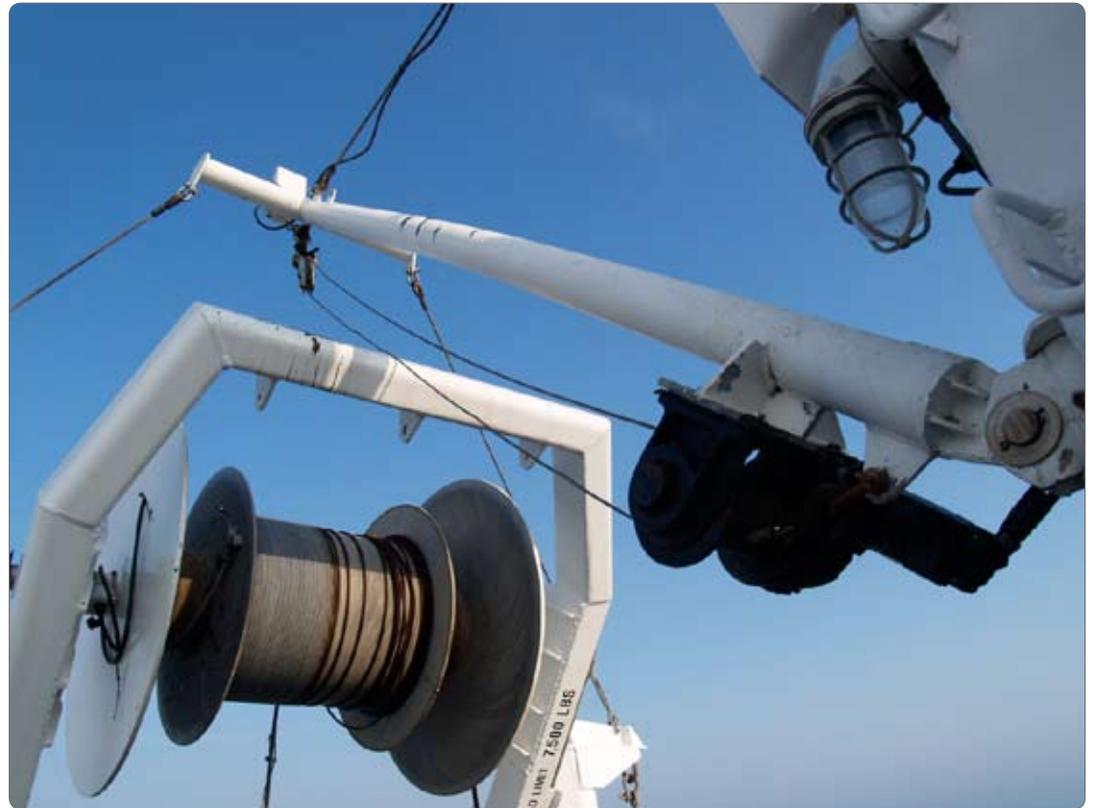
▲ **RIGGING** on the *R/V Dempsey*. The large net reel is used to deploy the rosette. The cable connecting the rosette to the net reel contains electrical conductors which allow the crew to see in real-time the data collected at each site.
