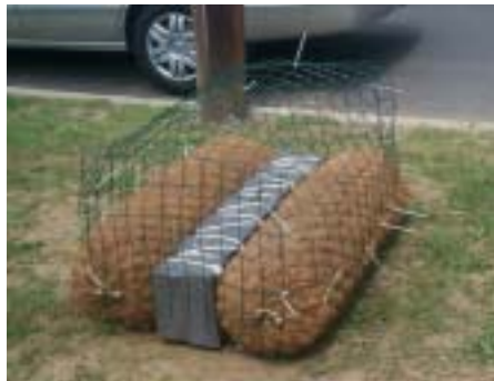
A unit of the floating wetland armature prior to planting. The gray material is high buoyancy foam. Coconut fiber "logs" on either side provide a planting substrate.
