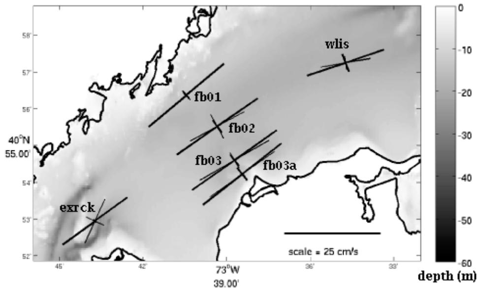
Figure 8. M2 tidal ellipses at 3m depth (heavy line) and near bottom (light line) for ADCP deployments in the western Sound. Semi-major and semi-minor axis amplitudes are shown centered at the location of the deployment.
