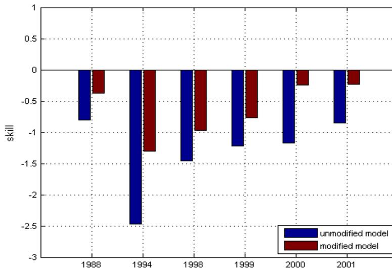
**Figure 30. Skill for the DO variable for the 6 years simulated using both the unmodified version of SWEM and the version with enhanced production and respiration, and realistic mixing.**
