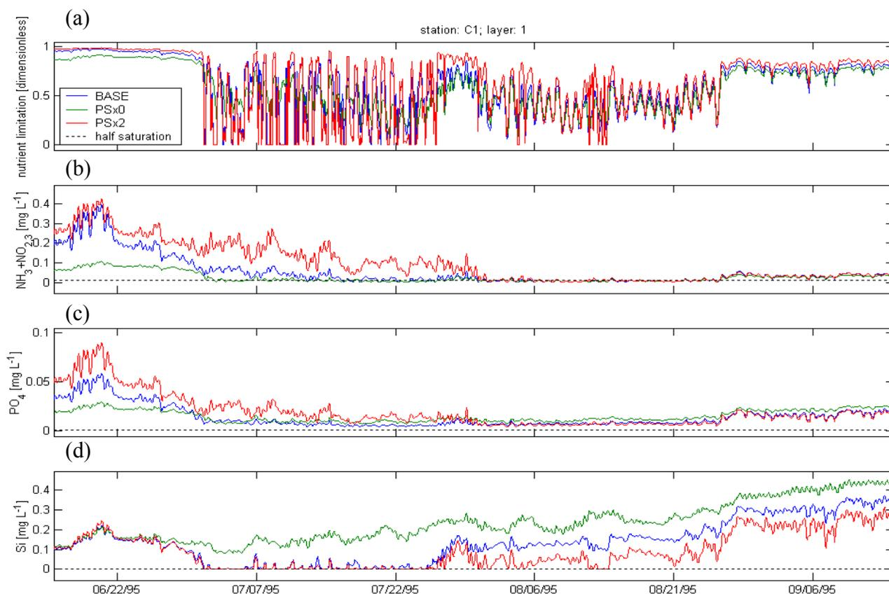
**Figure 20. June-September nutrient limitation for PHYT2 and nutrient levels with PS loading perturbations at station C1 (cell 41,50); blue: unchanged, green: no PS loading; red: doubled PS loading; (a) nutrient limitation factor, (b) organic nitrogen, (c) phosphate and (d) dissolved (available) silica.**
