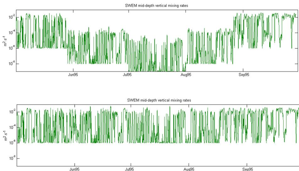
**Figure 12.** Comparison of the SWEM model predictions for the evolution of vertical eddy flux coefficient  $K$  ( $m^2/s$ ) near the CTDEP station B3 in the summer of 1995. (a) displays the vertical eddy diffusion coefficient at mid-depth and (b) with the ad-hoc reduction of the vertical eddy coefficient turned off.
