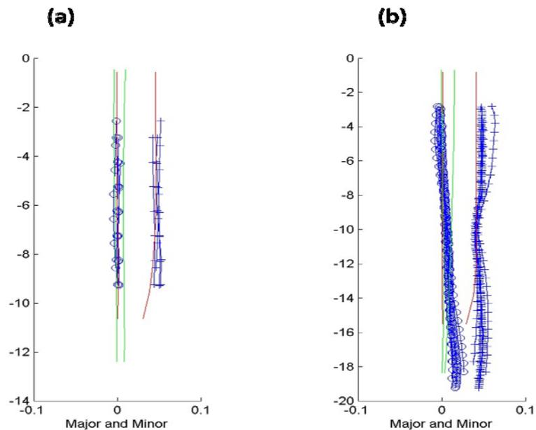
**Figure 10.** Comparison of the vertical structure of the M6 tidal current ellipse parameters from data (blue symbols) and the hydrodynamics module of SWEM (red lines). There are multiple profiles of observations because there were several deployments at each site. The green lines are from an alternative model that we do not discuss here. (a) and (b) show the major and minor axes (m/s) at stations fb02 and exrk.
