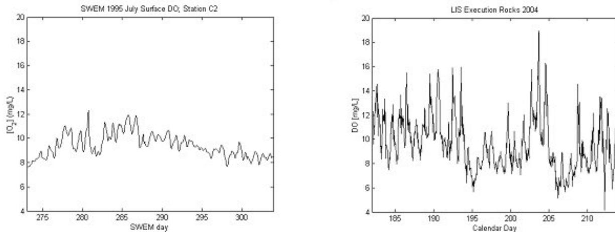
**Figure 23. (a) High frequency variation in DO at C2 in the July 95 SWEM simulation and (b), an example of the evolution at a buoy in the same vicinity (Execution Rocks) in July, 2004.**
