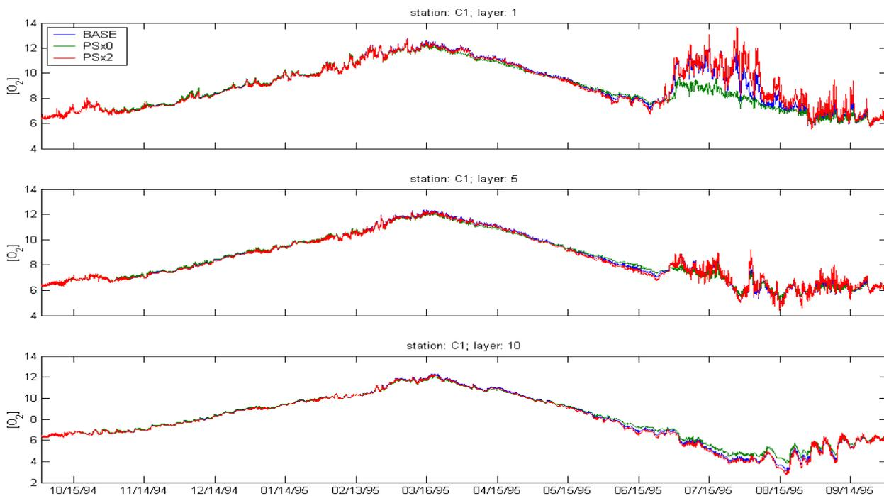
**Figure 19. SWEM PS loading perturbations at station C1 (cell 41,50); blue: unchanged, green: no PS loading; red: doubled PS loading; top panel: surface layer; middle panel: mid-depth layer; bottom panel: bottom layer.**
