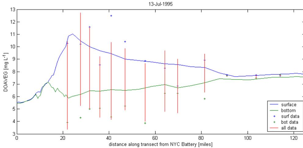
Figure 2. Comparison of the along Sound structure of the near surface (blue) and near bottom (green) DO concentration predicted by SWEM for July 1995. The surface and bottom observation of CTDEP are shown by the \* and + symbols respectively, and the range of the profile data is shown by the red lines.
