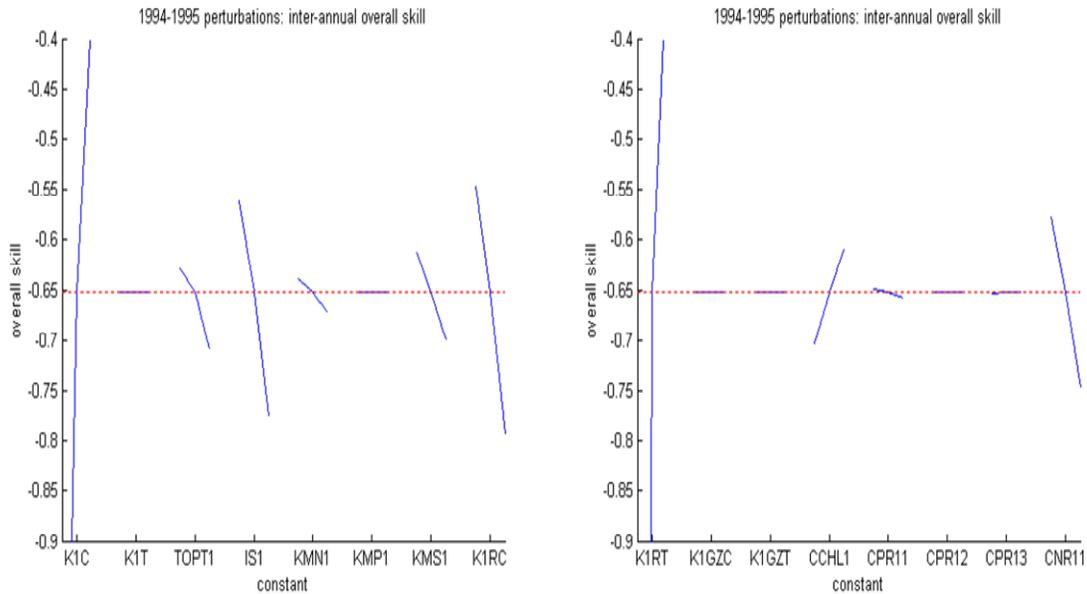
**Figure 16. Change in Skill,  $S_1$ , for the 1995 simulation resulting from changes to 16 model parameters and the 1995 simulation. The effect of increasing the parameter value by 10% is shown on the right side of each line segment and the effect of decreasing it is shown on the left.**
