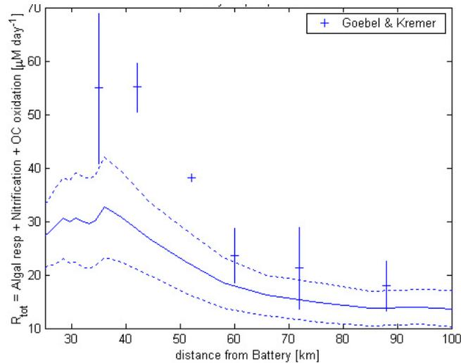
**Figure 22.** SWEM means (solid horizontal line) and standard deviations (dotted lines) of near surface (layers 1 and 2) July-August O<sub>2</sub> respiration rates ( $\mu\text{M day}^{-1}$ ) plotted by along-sound distance from the NYC Battery. Also shown by the vertical lines are the means and standard deviations of measurements by Goebel and Kremer (2007).
