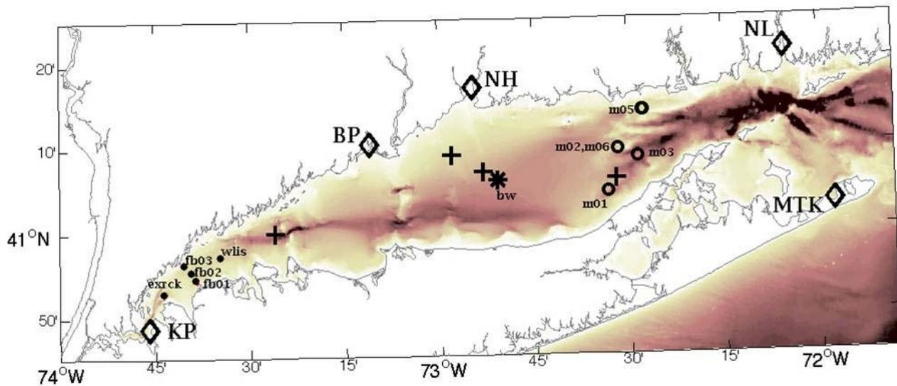
Figure 7. Bathymetric map of Long Island Sound. Diamonds show the location of NOAA tide gauges (KP = Kings Point, BP = Bridgeport, NH = New Haven, NL = New London, and MTK = Montauk), dots show LISICOS stations, asterisk shows central sound ADCP location, circles show LIS NSF stations, and pluses show historical current meter locations.
