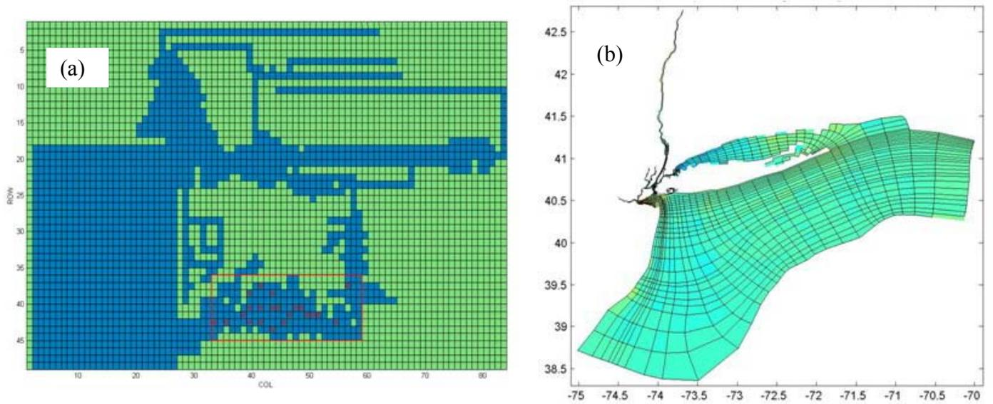
**Figure 5. (a) The SWEM domain with the land shaded in green and the ocean shaded blue. The cells that simulate LIS are within the red box. (b) A geographic representation of the geometry of the model grid.**
