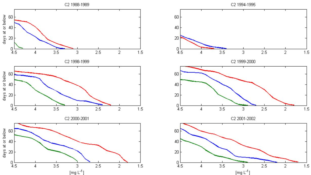
**Figure 29.** Duration the solution at station C2 falls below a threshold. The blue line represents the solutions obtained with the original SWEM code. The green curve shows the SWEM solution with mixing reinstated, and the red line show our modified model that includes increased respiration and vertical mixing.
