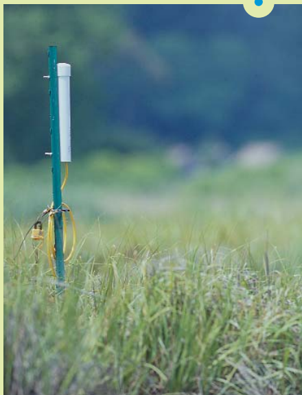
A water level recorder, right, collects hydrologic data.
