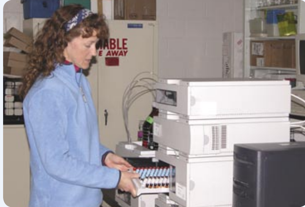
▲ A LAB TECHNICIAN loading sample vials into the automated High Performance Liquid Chromatograph.
