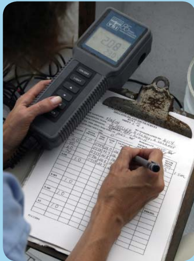
Recording water quality monitoring aboard the IEC research vessel Natale Colosi to document low dissolved oxygen conditions. Photo by Peter L. Sattler.
