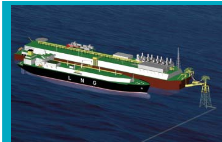
LNG carriers would dock at the proposed Floating Storage and Regasification Unit (FSRU) and offload the LNG as depicted in this artist's rendering. Courtesy of BroadwaterEnergy.com.
