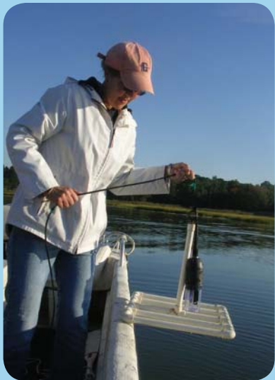
Friends of the Bay water quality volunteer Carla Panetta lowers a quanta sonde to measure the dissolved oxygen content, temperature, and salinity of the water in the Oyster Bay/Cold Spring Harbor Estuary. Photo courtesy of Friends of the Bay.
