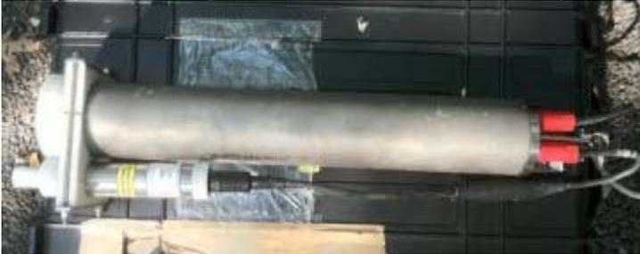
The Hydro C/CO<sub>2</sub> probe (Contros) attached to a boat for taking spatial measurement of CO<sub>2</sub> levels in Northport Bay during May 2012. Photo taken by Theresa Hattenrath-Lehmann.
