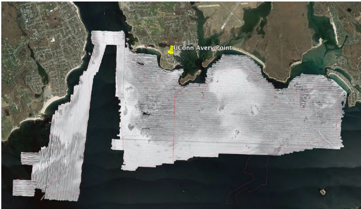
Figure 2.3-11. Mosaic of backscatter data from Survey Blocks 23, 24, and 25 generated by the Geoswath GS4 processing
