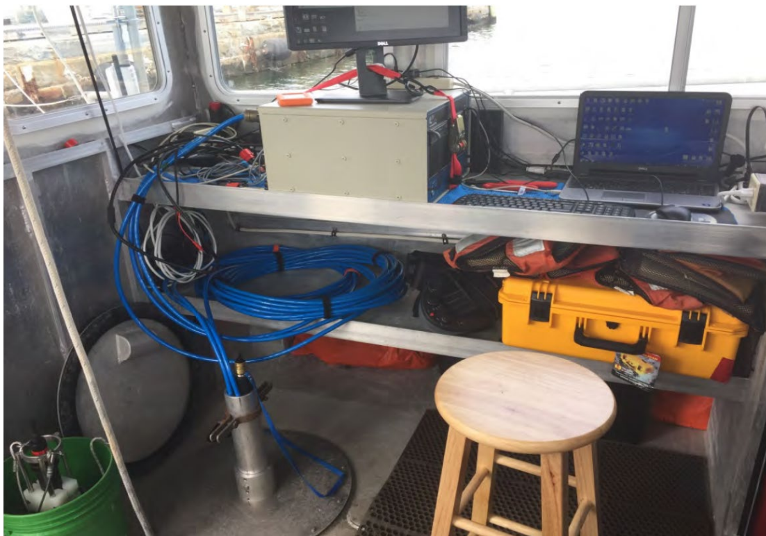
Figure 2.3-6. Geoswath setup on the R/V Weicker , moonpool cover is in the lower left
