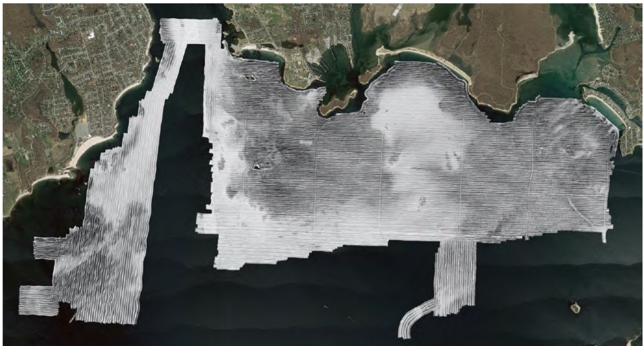
Figure 2.3-14. Mosaic of backscatter data from Survey Blocks 23, 24, and 25 generated by the CARIS processing
