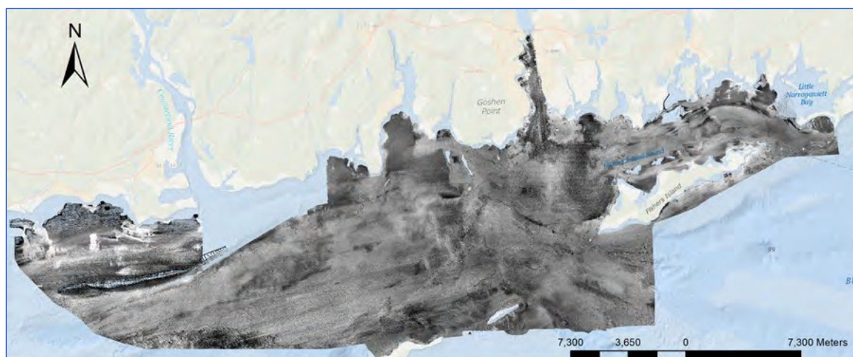
Figure 5.1-4. Acoustic backscatter mosaic of the Phase II study area that was used for seafloor characterization. Darker shades generally represent finer sediments; lighter shades generally represent coarser sediments.
