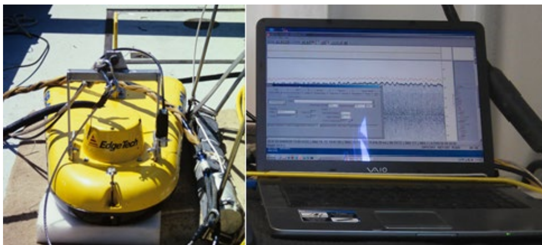
Figure 4.3-2. Lamont EdgeTech Chirp 424 subbottom profiler system (left) and EdgeTech Discovery software (right)
